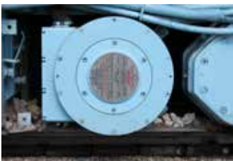
TM1200 continuous miner tram motor installed
