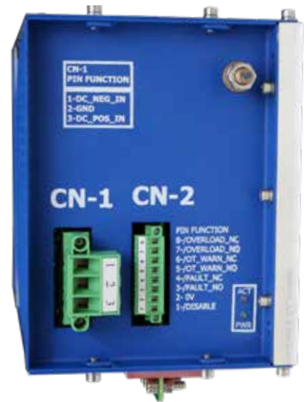
Power Supply input side
