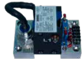
Ground Fault Diode/Relay (A800203)
